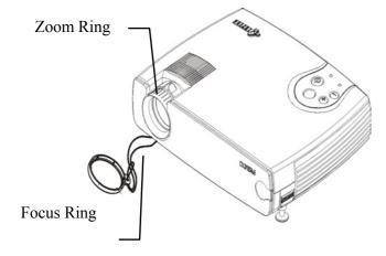
Rotate the zoom ring and focus ring until the projected image is clear and at the desired size. The projector can focus within the range of 5 feet (1.5m) to 33 feet (10m).
